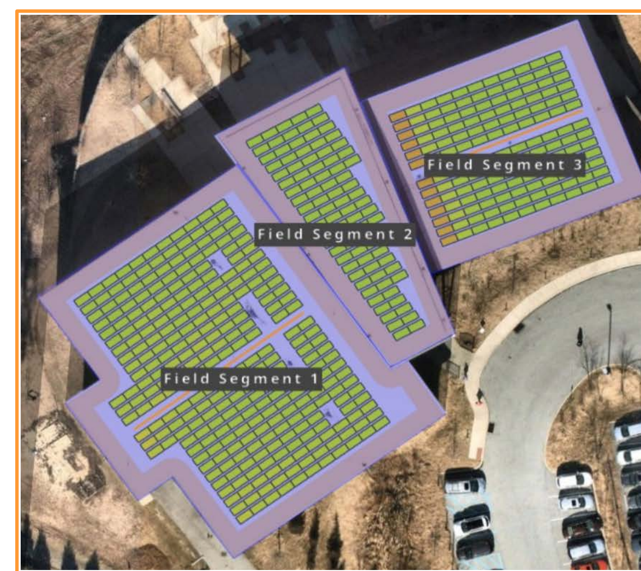
Fig. 3 Rooftop solar potential of the CREC The roof has an overall Solar access rating of 98.8% Courtesy of independence Solar
